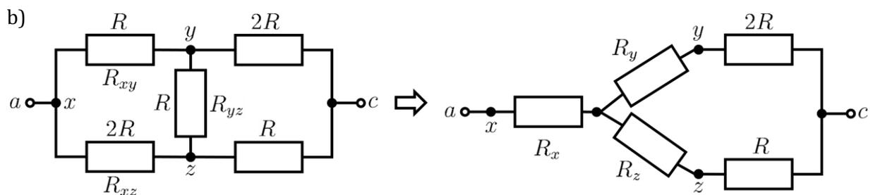
$$R_x = \frac{R_{xy}R_{xz}}{R_{xy} + R_{xz} + R_{yz}} = \frac{R}{2}$$
