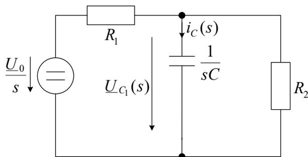
$$\frac{\underline{U}_{C_1}(s)}{\frac{U_0}{s}} = \frac{\frac{\frac{1}{sC}R_2}{\frac{1}{sC} + R_2}}{R_1 + \frac{\frac{1}{sC}R_2}{\frac{1}{sC} + R_2}} = \frac{R_2}{sCR_2R_1 + R_2 + R_1}$$
