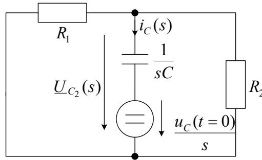
$$\frac{1}{s+c} \text{ wobei } c = \frac{R_1 + R_2}{CR_1R_2}$$
