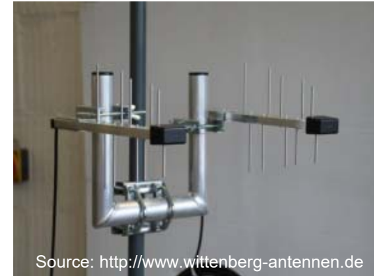
2-element Yagi for LTE800
